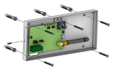
For optimal performance of the wireless system the Air2-BS200 transceiver module must be located at the core of the wireless network and area of use of remote-control keys, in a placement which allows easy connection of the I-BUS cable to the control panel.
