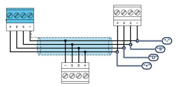
The peripheral devices of Inim Electronics control panels are to be connected to the control panel via the I-BUS.
