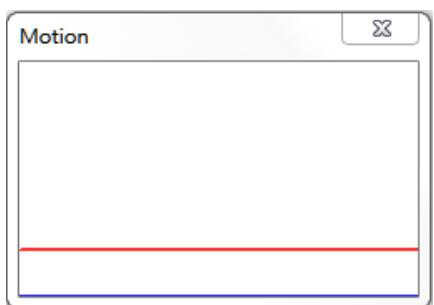
When motion is detected, the signals will be displayed on the Motion window as shown below. Motion is detected by comparing sampling pixels in the detection area of two consecutive live images.
